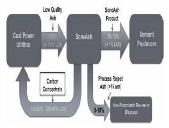
At the heart of the SonoAsh process is the Sonicator, which enables the extraction and gradation of ASTM C618 fly ash from previously landfill- or impoundment-grade coal combustion residuals.
