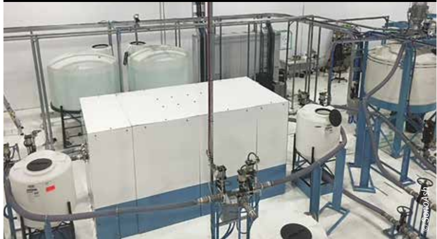
The Sonoash Sonicator reactor can process a broad range of coal ash samples
